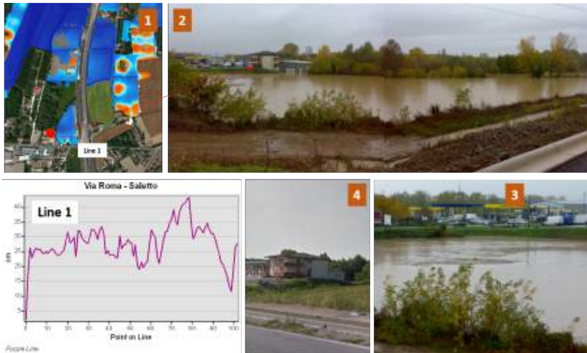
Figure 52 1) Flood depth on November 3 rd in Via Roma in the Saletto area of interest; 2-3) pictures taken by civil protection on November 2 nd at 9:30 am local time; 4) Google Street View of the same area; bottom left: flood depth profile along the line in box 1
