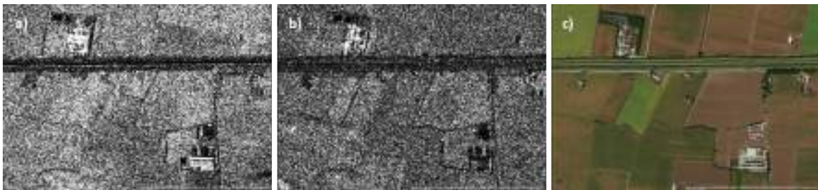
Figure 32 In a) and b) the same area is observed with different incidence angle and it can lead to false alarms due to the different radar shadow.
