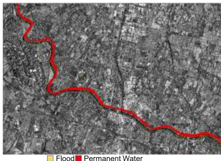
Figure 19 An error in CIMA foundation map of 6 th November 2010. Flood area (in orange) are reported over permanent water bodies, in this case a river. In red, pixels labelled as permanent water in CIMA's map. It is clear that these are shifted compared to the SAR data, indicating that probably an external layer for water bodies was used. These errors are affecting the results in the confusion matrix.
