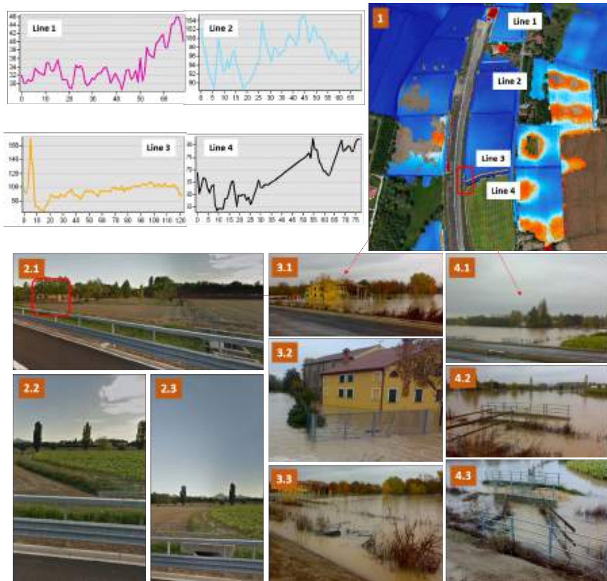
Figure 53 1) Flood depth on November 3 rd along the new motorway crossing Saletto area; 2) Google Street View images of the areas in boxes 3 and 4; 3-4) Images taken on November 2 nd at 9:30 pm; Top left: flood depth profiles along the lines in box 1
