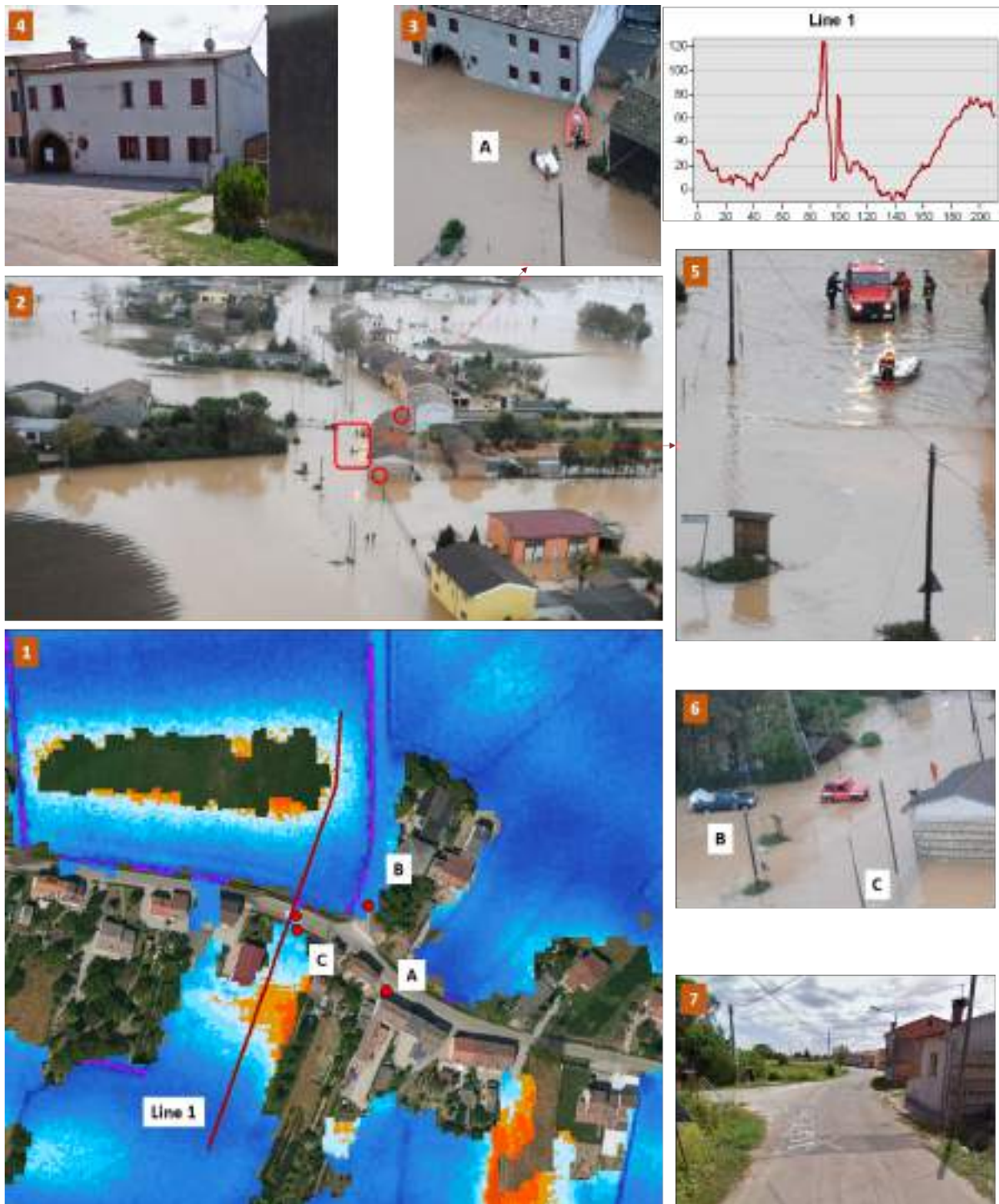
Figure 50 1) Flood Depth on November 3 rd over Cabriani area in the Saletto area of interest; 2-3-5-6) Aerial views of the flood taken on November 1 st at 16:30 local time; 4-7) Google Street View corresponding respectively to image 3 and 6; top right: flood depth profile of line 1 shown in 1)
