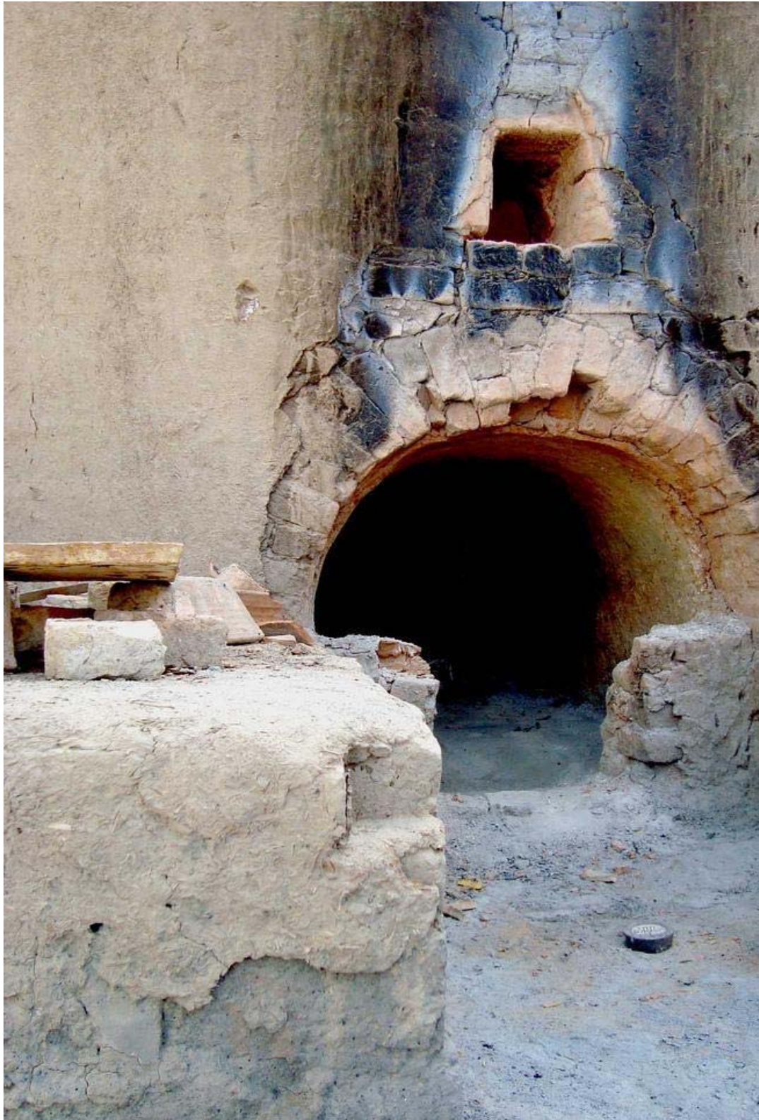
Fig 25. The furnace for baking the pottery at a workshop in Hala.
