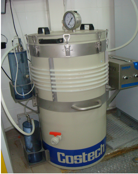
Figure 2.11: Dynamic Respirometric Index reactor.
