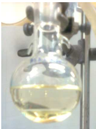
Figure A.3.27. Reaction mixture before reaction . Upper layer: P8,8,8,1NO 3 + Anisole; lower layer: aqueous HCl
