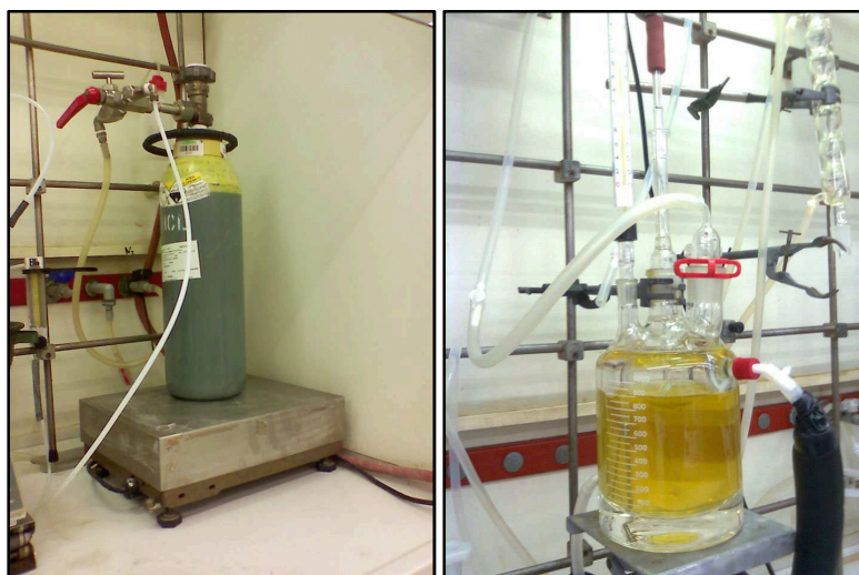
Figure 5.13 Pictures took during the scale up tests in Galentis. Hydrogen chloride cylinder (left) and a coated 1 L reactor (right) are shown.
