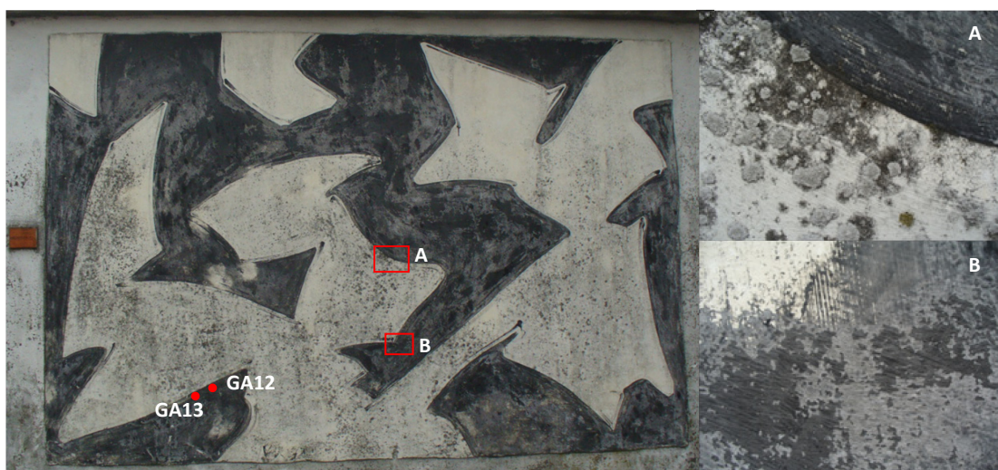
Fig. 4.1-1: Asdrubali' s mural as it looks today. A and B: enlarged details documenting the condition of the mural. The red dots mark the sampling points.
