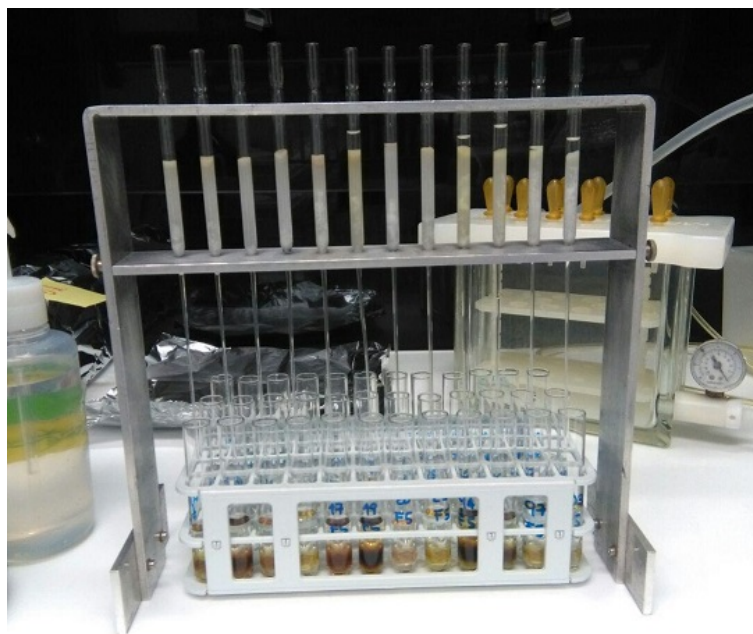
Figure 3.6: Clean-up of Hala Hu DCM-TLE with Pasteur pipettes filled with silica gel.
