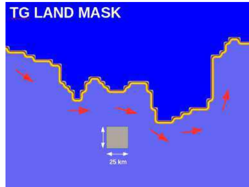
Figure 4.24: Totten Glacier area in NEMO land-sea mask. The NEMO simulated TS profile has been extracted from the gray box area that corresponds to a 625 \text{ km}^2 area. The box contains 16 grid nodes and thus as many vertical profiles of temperature and salinity. The red arrows indicate the simplified averaged horizontal ocean circulation.
