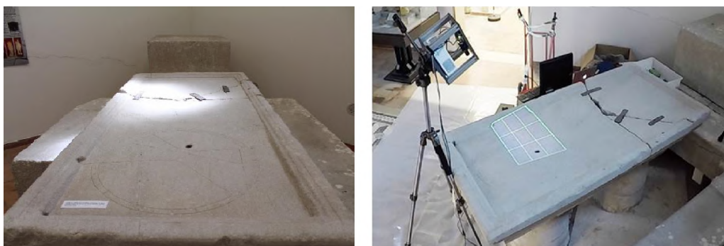
Figure 9.1: Left: Inscriptions on the top surface of the Euporus sundial. Right: 3D acquisition of the sundial: on the left the structured light scanner mounted on a tripod.
