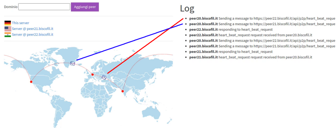
Figure 30: Monitoring page displaying some messages exchanged between servers. The red lines represent of the connections between three servers rented in India, California and Germany. This interface was provided by the German server.
