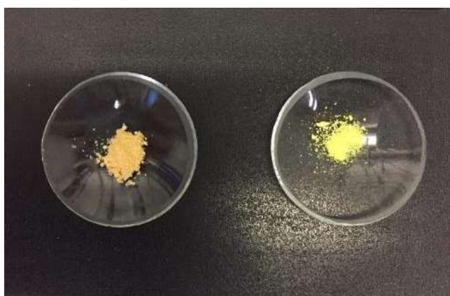
Figure 57. Two types of solid obtained at the end of the purification stage. On the left (darker one, RTPx-1), the solid left in the round bottom flask can be observed, while on the right (lighter one, RTPx-2) the solid remained at the bottom of the beaker is shown.
