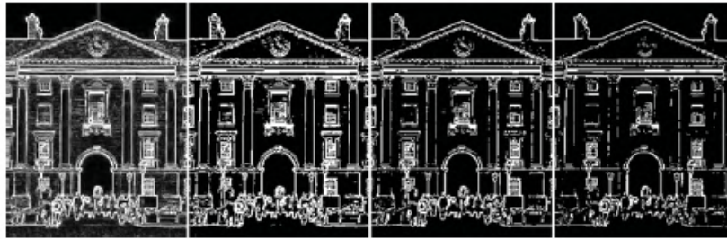
Figure 19: An edge gradient image (a) together with three thresholded versions (b), (c) and (d) thresholded at 120, 160 and 200 respectively
