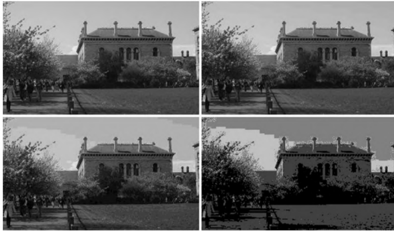
Figure 13: Four different quantizations of the same grey-scale image; top left 8 bits, top right 6 bits, bottom left 4 bits and bottom right 2 bits
