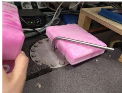
Figure 5.33: Stainless steel chamber with the lid placed on the getter line.
