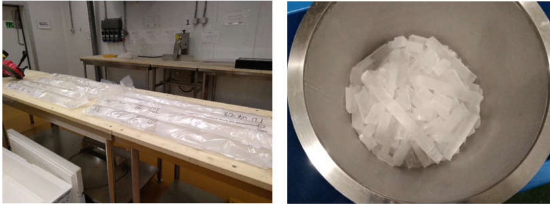
Figure 2.32: Left. ^{81}\text{Kr} dating samples preparation at the EuroCold facility at the University of Milano-Bicocca. Right. Cut ice samples ready for the air extraction at LSCE (France).
