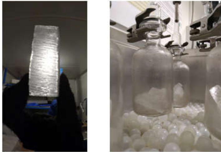
Figure 2.24: Left. Ice samples cut in the cold room. Right. Ice samples placed in the flasks before the melting step.
