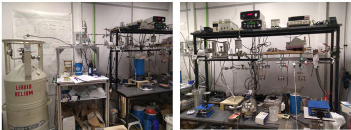
Figure 5.35: Getter method extraction line at LSCE. Left. Air transfer from the ice chamber to the dip tube. Right. Getter step.
