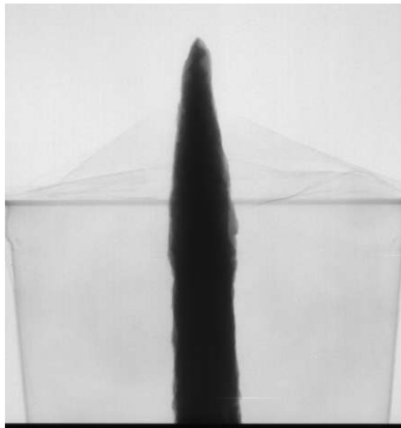
Figure 3.12: 2D radiograph of the javelin tip
