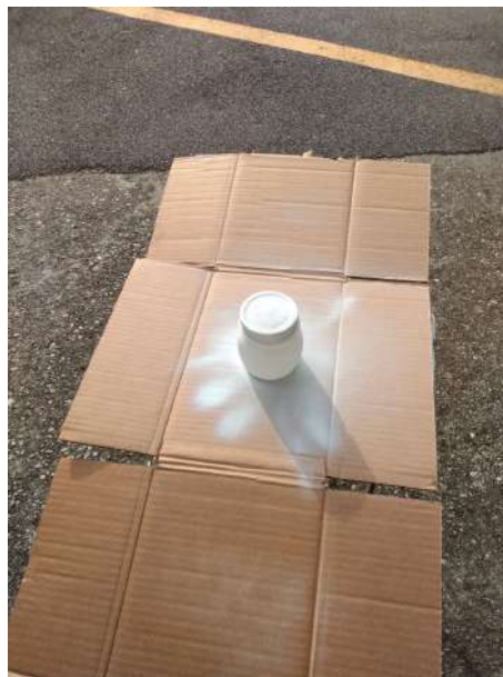
Figure 3.2: Example of transparent jar dusted with anti-glare spray (experiment made at the FabLab in Castelfranco Veneto)
