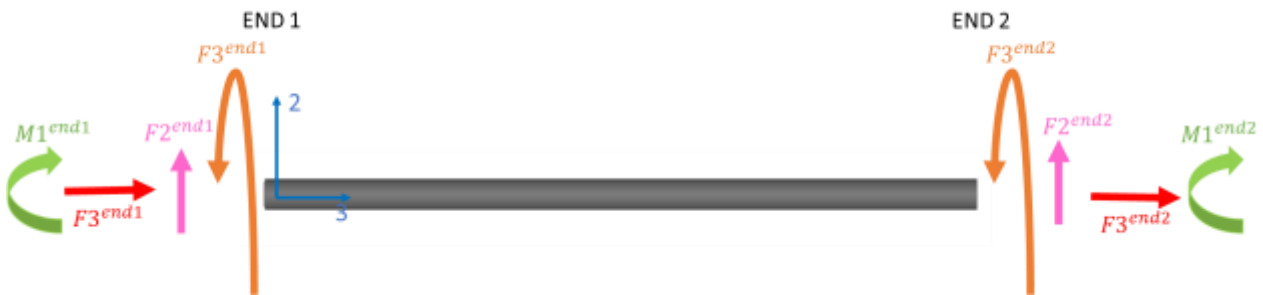
Figure 64. Beam node forces
