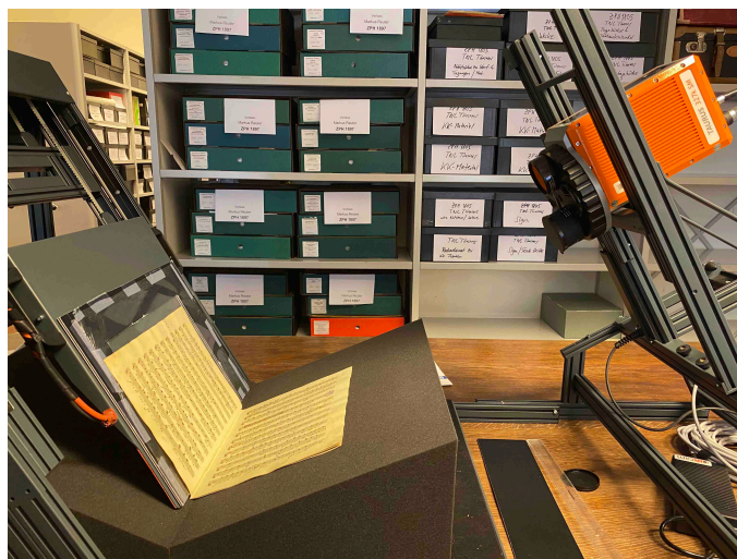
Fig. 9 - The manuscript is positioned on the copper plate ready to be reproduced by the thermographic camera.
