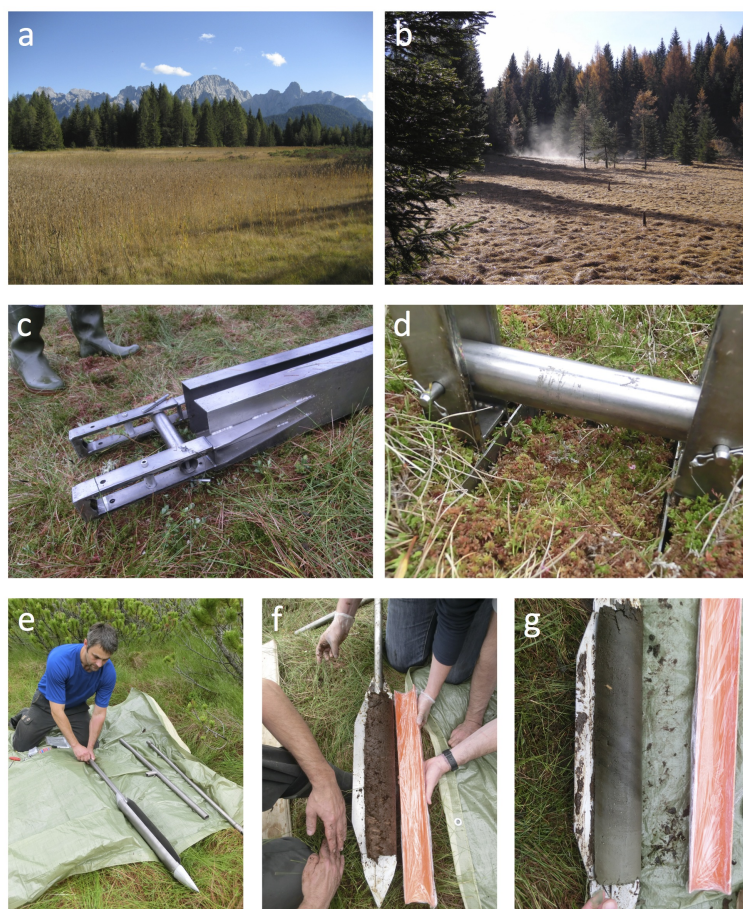
Figure 6.2: Val di Ciampo peat bog, as spring (a) and as autumn (b). Wardenaar corer (c-d). Panel (d) shows the high Wardenaar corer capacity of no-compressing during sampling. Belarus corer (e-g). Panel (f) is a picture of a middle core section collected with the Belarus corer, panel (g) shows the final section of the entire core with layers of lacustrine origin.
