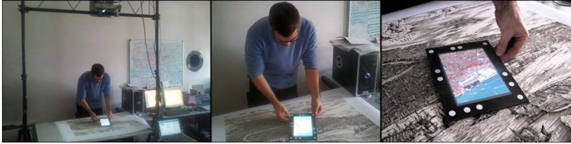
Figure 3.15: Actual setup and examples of usage by moving the controller above the printed map.
