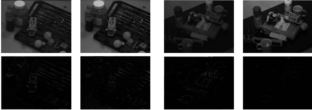
Figure 10.3: Shading (top-row) and specular factors (bottom-row) obtained for the same sample image pairs shown in Figure 10.2.
