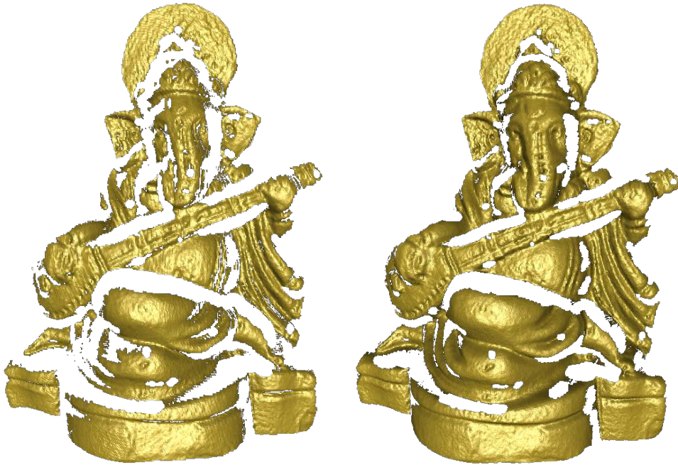
Figure 8.7: Reconstructed range-map triangulated from the OpenCV calibration and rectification (Left) and our proposed method (Right).
