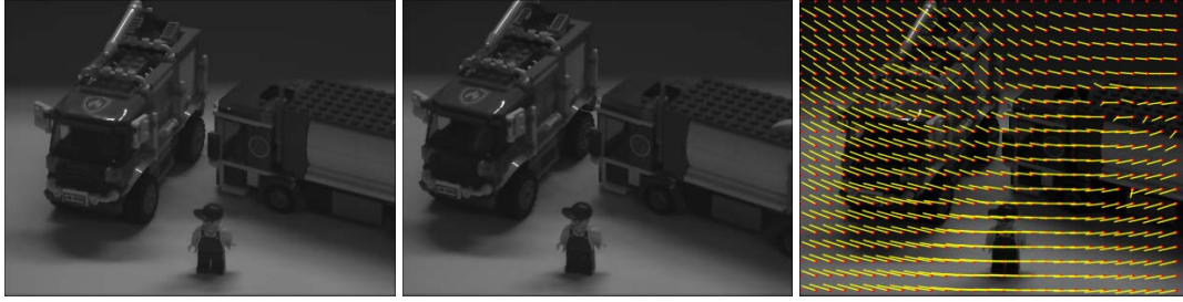
Figure 2.7: An example of optical flow estimation from two images (Left and Center) taken from a moving camera. At each point of the first image is associated a displacement (flow) vector to the corresponding point on the second.
