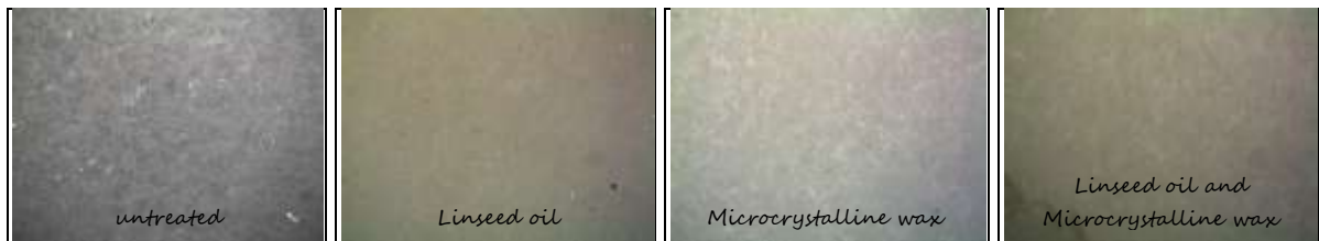
Figure 9.1: Micrographs of Carrara marble samples untreated, treated with linseed oil, microcrystalline wax, and linseed oil-microcrystalline wax at zero time. Long side images 6.78 mm.
