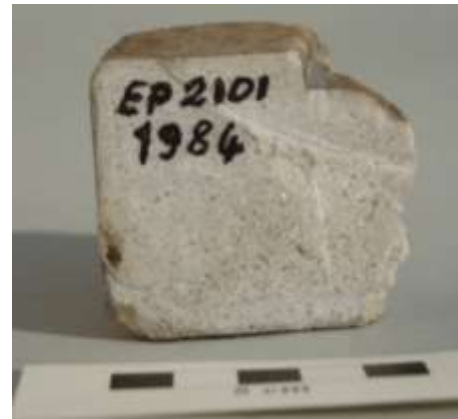
Figure 7.15: Specimen of Proconnesian marble from S. Marco Basilica treated in 1984 using EP2101.
