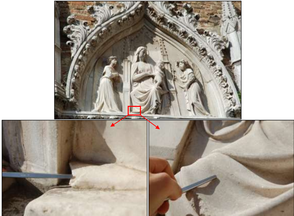
Figure 4.37: Sampling of a micro-fragment from lowest left part of the mantle of the Virgin Mary, adjacent to a previous broken area
