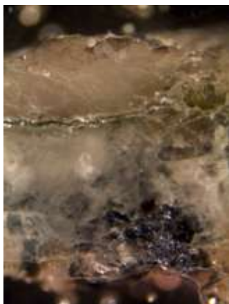
Figure 7.14: Micrography of CVM01 cross-section. OM. long side image 1.03 mm.
