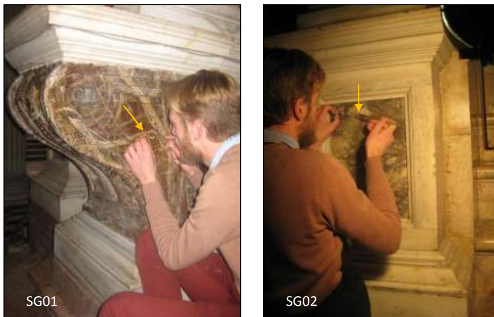
Figure 9.11: Sampling of superficial dark patina from different areas on the High Altar
