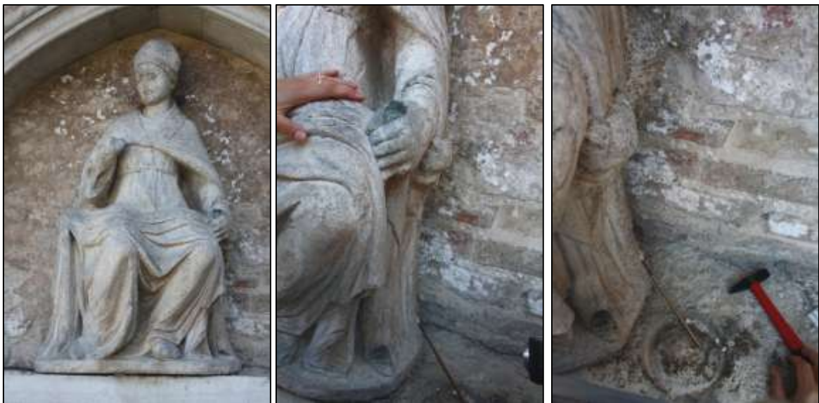
Figure 4.30: Sampling of a micro-fragment from the right side of the statue, close to the base.
