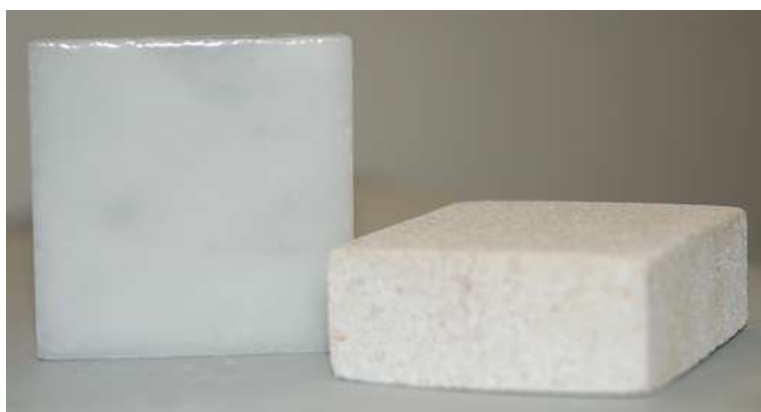
Figure 2.1: Carrara marble and Vicenza white limestone specimens
