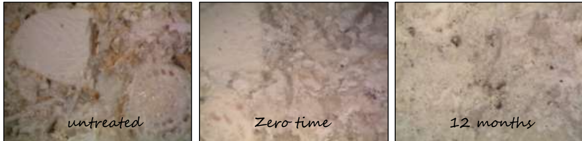
Figure 3.1: Micrographs of the same area of Vicenza white limestone untreated, treated with Ba(OH)_2 at zero time and after 12 months of outdoor exposure. Long side images 6.78 mm.
