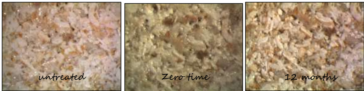
Figure 5.2: superficial aspect of untreated Vicenza limestone specimen, treated with PF3 at zero time and after 12 months of outdoor exposure. Long side images: 6.78 mm.
