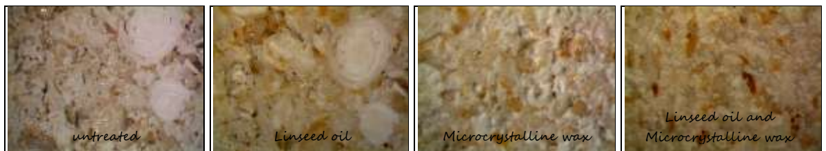
Figure 9.2: Micrographs of Vicenza limestone samples untreated, treated with linseed oil, microcrystalline wax, and linseed oil-microcrystalline wax at zero time. Long side images 6.78 mm.
