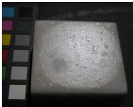
Figure 7.7: Picture of the imprinting of the sponge, during sponge test, on Carrara marble surface.
