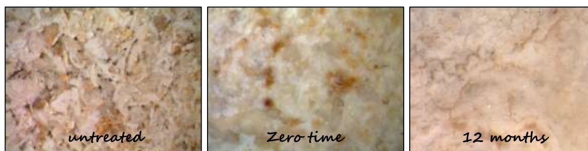
Figure 7.5: micrographs of the same area of Vicenza white limestone untreated, treated with EP2101 at zero time and after 12 months of outdoor exposure. Long side images 6.78 mm.
