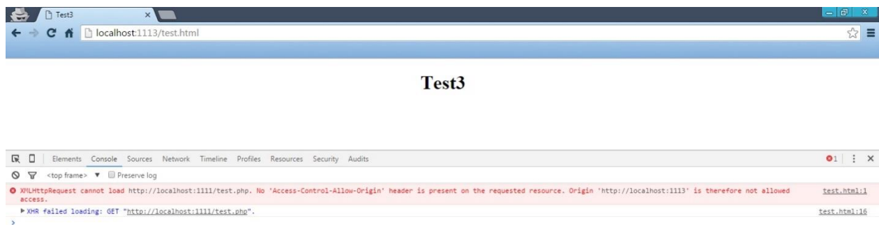
Figure 4.6: CORS Response of Client in origin 1113 using Console tab
