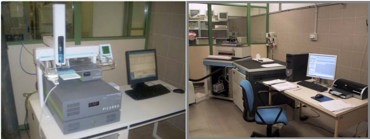
Fig. 5.6-1 Picarro L1102- i liquid analyzer with HTC PAL autosampler (on the left) and Thermo-Fisher Delta Plus Advantage with the 24-vial HDO device (on the right)
