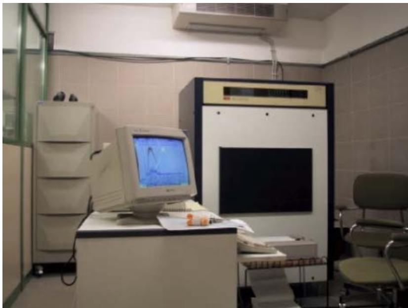
Fig. 5.6-3 The Wallach L.K.B. Quantulus liquid scintillation counter
