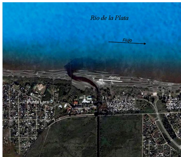
Figure 3.2.2.: Satellite image showing the littoral drift in the coastal zone of Río de La Plata
