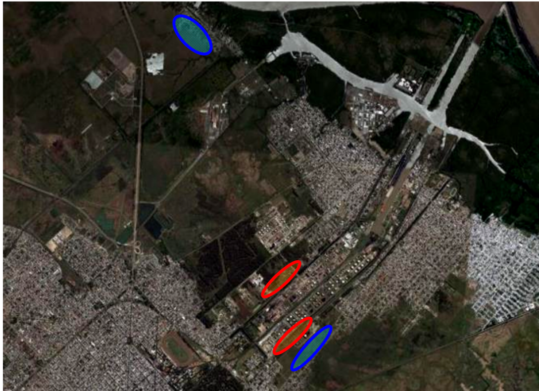
Figure 4.1.7 Profiling survey areas. Natural ground (blue) and anthropic fill (red)
