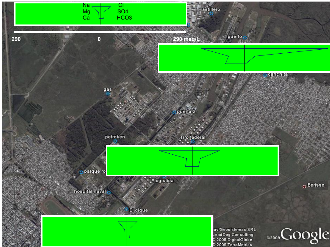
Fig. 4.6.9 Graphical representation by modified Stiff diagrams (Custodio, 1965) of the different types of water found in Puelche aquifer
