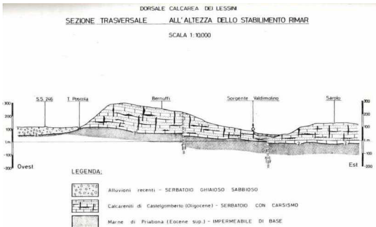
Figure 2.7: WE stratigraphic profile at the level of Rimar factory [from IRSEV study]
